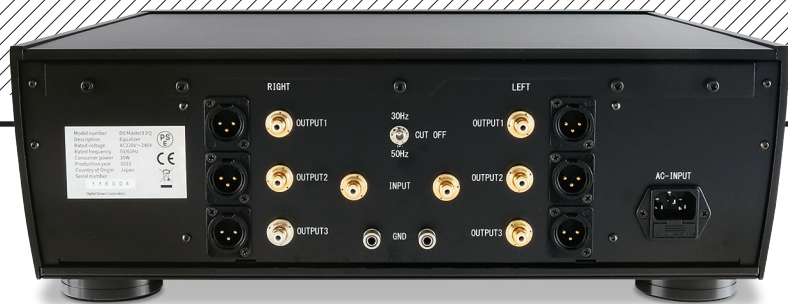
ABOVE: The PSU/equaliser provides power for the pick-up's internal LEDs via the input RCAs [centre]. The outputs, on RCAs and XLRs, offer different levels of bass boost from two alternative - 30Hz and 50Hz - turnover frequencies [see Graph 1, opposite]
